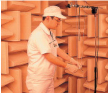
Anechoic room supports quality development of noiseless mot
